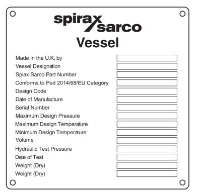
Fig. 2 Typical FV type flash vessel name-plate details
