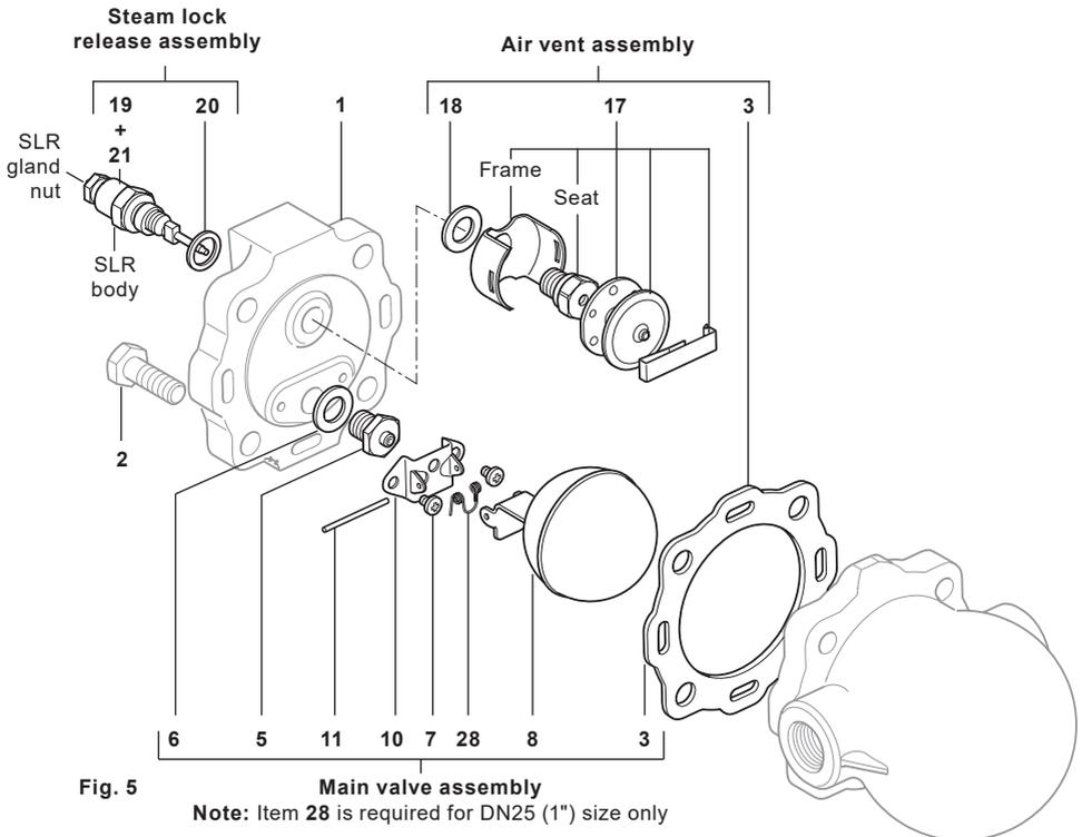
FTGS14 Ball Float Steam Trap DN15 (½") to DN25 (1")
