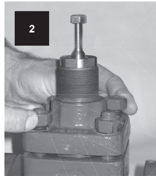
Finger tighten opposing bonnet nuts or bolts evenly in pairs.
