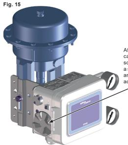
After manually screwing the cap  $\rm Ex\,d\,M50$  cap, loosen the  $\rm Ex\,d\,locking\,cap\,M5\,x\,10$  screw, using a 4 mm allen key, by exerting a slight pressure between the screw head and  $\rm EX\,d\,cap$ . This operation is to prevent accidental unscrewing of the  $\rm Ex\,d\,cap$ .
