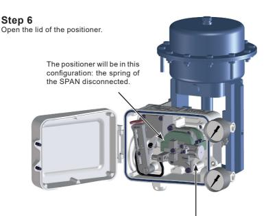
Fig. 16 Turn the ZERO dial (the green one), until the valve is opened at 50%
