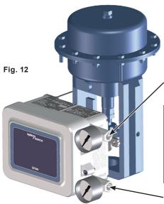
Connect the pneumatic output of the positioner to the actuator
