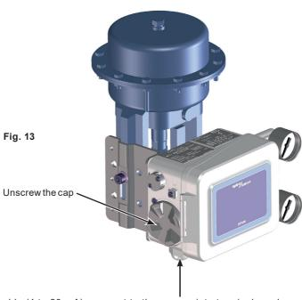
Insert the electric cable (4 to 20 mA), connect to the appropriate terminals and screw the cap.
