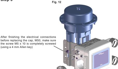
before replacing the cap, M50, make sure the screw M5 x 10 is completely screwed (using a 4 mm Allen key)
