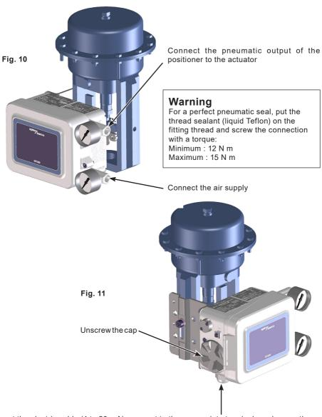
Insert the electric cable (4 to 20 mA), connect to the appropriate terminals and screw the cap.
