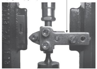
Depending on the travel of the valve actuator and depending on the actuator yoke, apply a medium strength thread locker to the sliding pin and screw into the correct hole on the sliding pin holder and tighten. Use Figure 7 and Table 1 to determine the correct hole to use.
