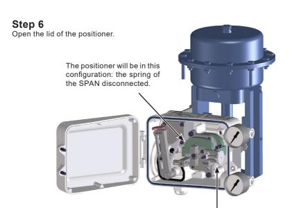
Fig. 14 Turn the ZERO dial (the green one), until the valve is opened at 50%
