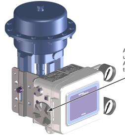
After manually screwing the cap M50, unscrew the screw M5 x 10 (using a 4 mm Allen key, creating a slight pressure between the screw head and stopper M50
