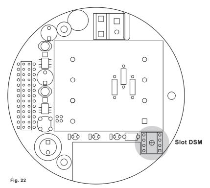
At any exchange watch the polarity of the memory chip. Pin 1 is signed by a dot or a notch.
