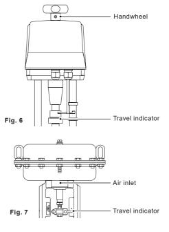
For the pneumatic actuated control valve, remove the existing air supply and connect an independent air supply to the actuator (pressure not to exceed 6 bar g (87 psi g)), allow the valve to fully open, remove the air supply from the actuator allowing the valve to close. Reconnect the original pipework (Figure 7).
