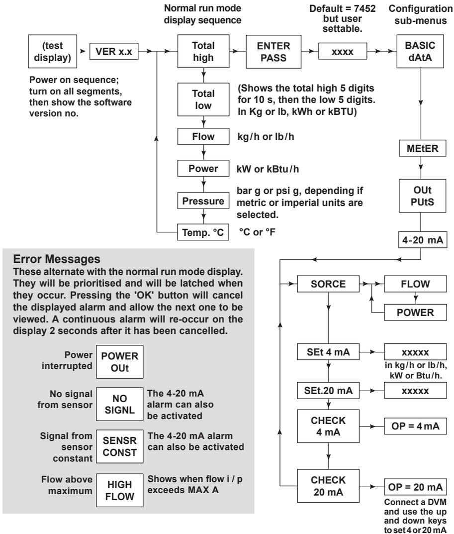
From the Basic dAtA menu navigate to OUTPuTs and press the right arrow to enter the sub menu of 4 - 20 mA.
