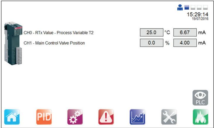
**Fig. 58** Analogue retransmission outputs
