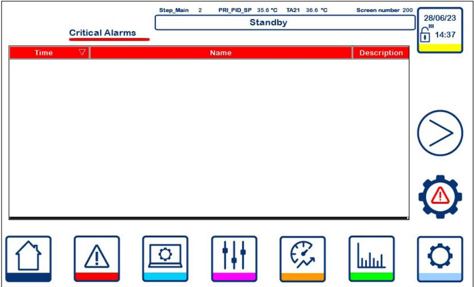
The notifications displayed on the Critical Alarms screen (200) are displayed to inform of the package not running within specification.
