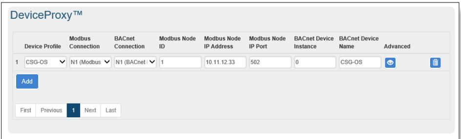
Once the device profile has been loaded, use the Save button to restart the module with the new settings loaded.
