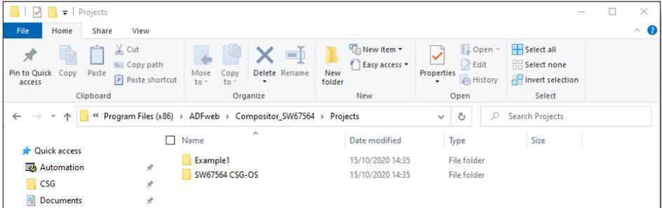
Open the software and load the SW67564 CSG-OS configuration. The 'Set communications' button will allow users to edit the settings for the external connection.
