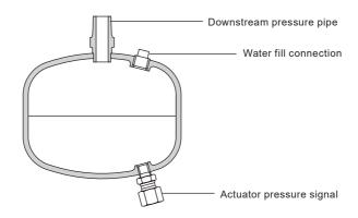
Fig. 2 Water seal pot - WS4/WS4-3
