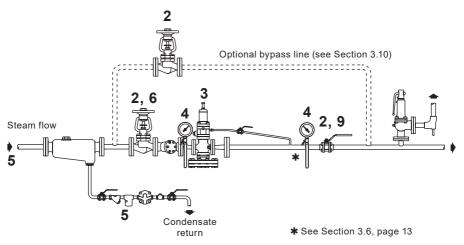
Fig. 8 Setting procedure sequence DP27, DP27E and DP27Y
