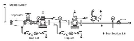
Fig. 6 Two pressure reducing valves installed in series
