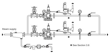
Fig. 5 Two pressure reducing valves in parallel
