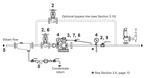
Fig. 9 Setting procedure sequence DP27R
