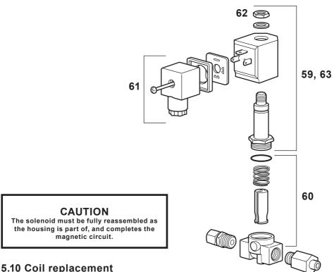
Switch off the electrical power supply and disconnect the coil lead wires.
