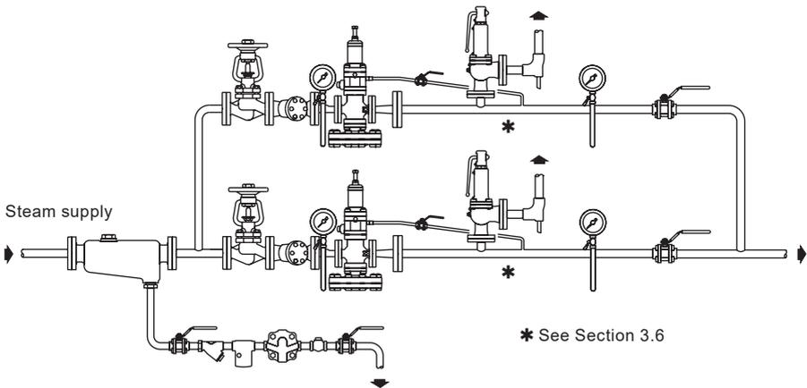
Fig. 5 Two pressure reducing valves in parallel
