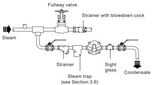
Fig. 2 Recommended installation
