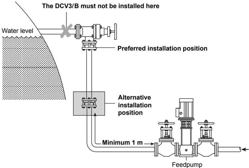
**Note:** The illustration shows preferred and alternative installations for the DCV3/B boiler feed check valve (mounted between flanges).
