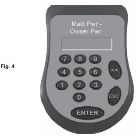
Insert the digit 3 and confirm by pressing the ENTER key.
