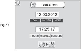
To change date or time settings, press the corresponding key (DAY/MONTH/YEAR or HOURS/MINUTES/SECONDS), enter the new value using numerical keypad displayed and confirm by pressing the **RET** key. The new value will now be displayed on the screen.
