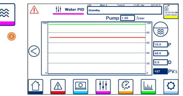
Water PID settings (420) also includes the pump offset value and a live PID graph showing the process and control values, and the process set-point.
