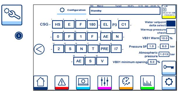
System configuration (780) allows Spirax engineers to alter the configuration of the CSG-HS set during the commissioning sequence (only available in standby mode).
