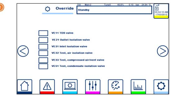
Digital override (750) open and close fitted and available isolation valves (only available in standby mode)
