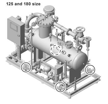
Ring-nut for extraction/withdrawal of mounting foot
