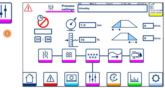
Main process set-points (400). Including clean steam pressure, water level, ramp up time and ramp down time.
