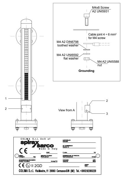
Do not remove or tamper with the connection between the instrument scale (1) and the nameplate bracket (2).
