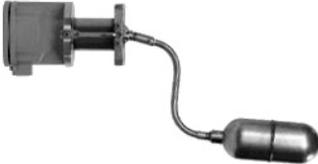
Type recommended in applications containing foam, inclusions and viscous fluids, where conditions require that the fulcrum point is not in touch with the process liquid.
