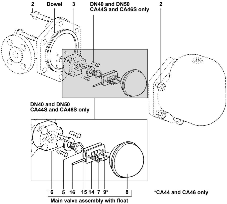
Fig. 6 CA44S and CA46S DN40 and DN50
