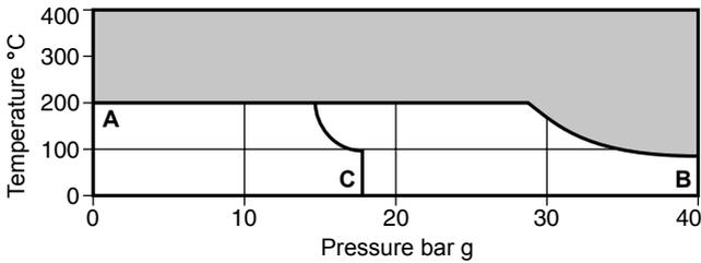
**CA46S - DN15, DN20 and DN25 flanged**
