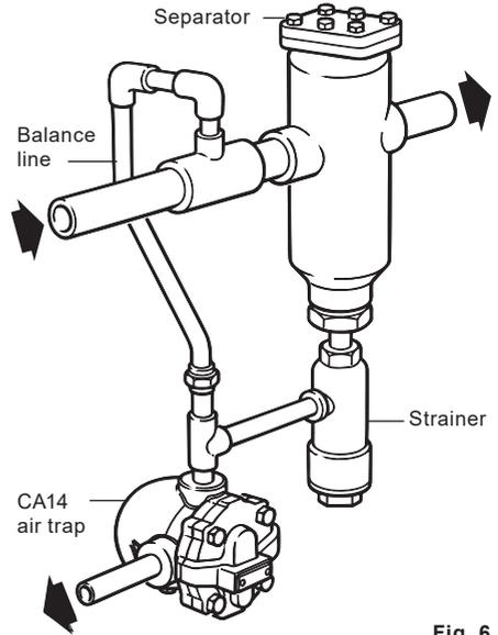
Fig. 6 Air trap draining a separator on a compressed air main
