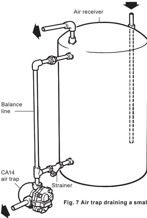
Fig. 7 Air trap draining a small receiver
