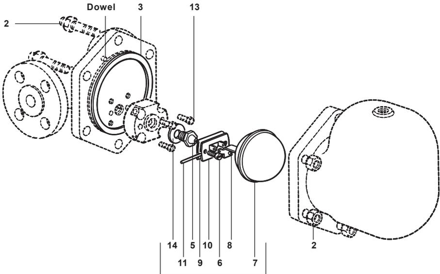
Main valve assembly with float
