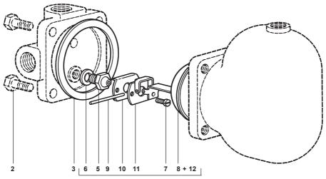
Main valve assembly with float Fig. 9
