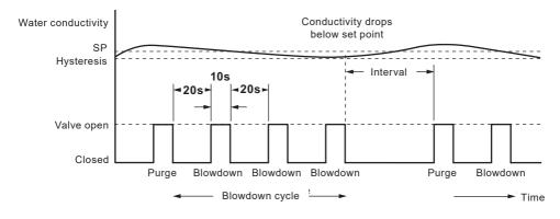
Fig. 21 ON/OFF control with purge and pulsed output
