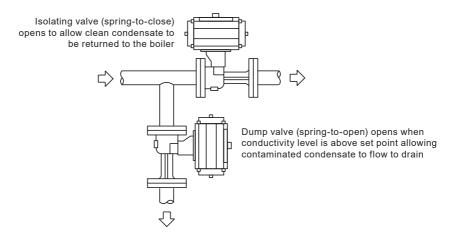
Fig. 7 CCD system showing alternative arrangement of seperate valves
