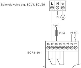
Fig. 13(a) BCV1, BCV20 and solenoid valves
