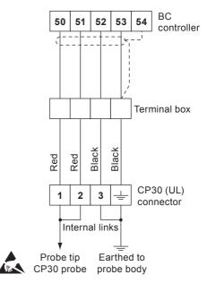
Fig. 25 Alternative wiring for the UL version
