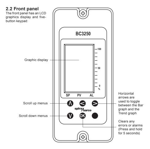
Fig. 1 Front panel keypad and definitions.
