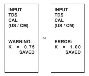
**Note:** If the calibration is accessed via the commissioning mode, the input voltage from the probe circuit is displayed during 'CAL ..'. This ranges from 0 - 2.500 V and is used for diagnostic purposes. The valve varies with conductivity, temperature and probe condition / installation.
