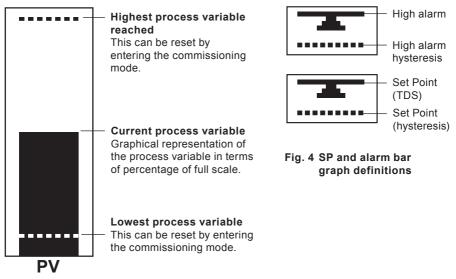
Fig. 3 PV (conductivity) bar graph definitions
