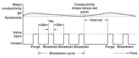
Fig. 8 Pulse output with purge time set (>0s)
