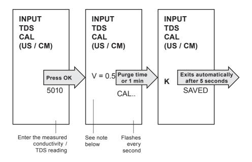
If the cell / probe factor is outside normal range (0.20- 0.70), 'WARNING' will be displayed. If the cell / probe factor is excessive (< 0.01 or > 1.00), 'ERROR' will be displayed. See Section 9, Fault Finding.
