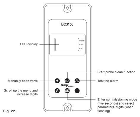
The product has no battery. The programmed settings are held in non-volatile memory (Flash) and are written to after changing a parameter and pressing the **w** button.
