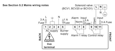
Fig. 15 BCV1, BCV20 or BCV31 solenoid valves
