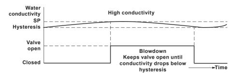
Fig. 2 Continuous output (purge time = 0s)
