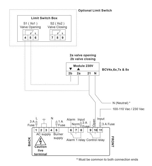
Fig. 19 BCVxx Blowdown valves with 100-110 Vac / 230 Vac Supply 1 cable / 2pt
