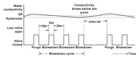
Fig. 4 Pulse output with purge time set (>0s)
