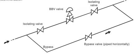
BBV Automatic or Manually Actuated Boiler Blowdown Valves
