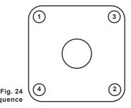
DN15 - DN50 bonnet tightening sequence
