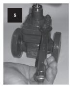
Using a torque wrench lightly and evenly tighten each bolt or nut by 45°, following the sequence illustrated in Figure 24, page 48.
