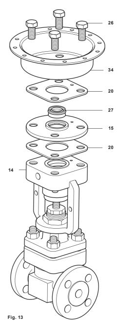
BBV Automatic or Manually Actuated Boiler Blowdown Valves
