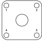
Fig. 16 Bonnet tightening sequence
