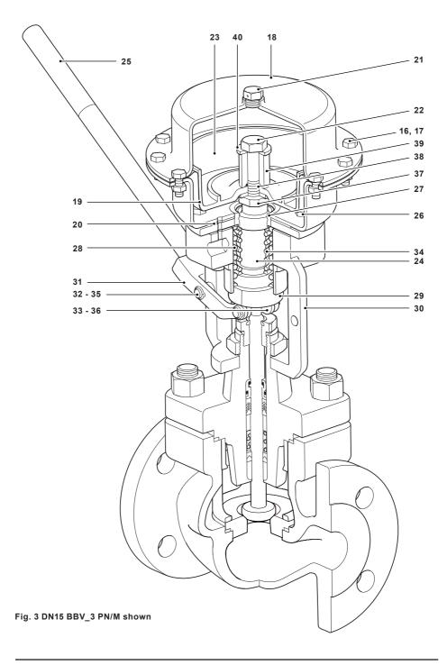
BBV Automatic or Manually Actuated Boiler Blowdown Valves
