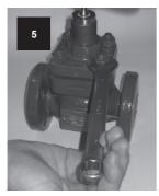
Using a spanner lightly and evenly tighten each bolt or nut by 45°, following the sequence illustrated in Figure 5, page 40.
