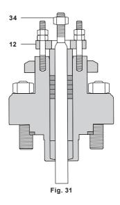
BBV Automatic or Manually Actuated Boiler Blowdown Valves
