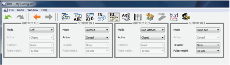
Four relay outputs can be configured.
