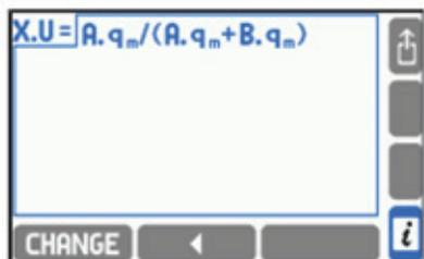
Unit of calculated result should be written in a text form (up to 6 characters). In the mass flow rate formula units cannot be deactivated in calculations (see Section 10.5.3).
