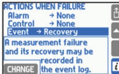
The date and time of each event occurrence is recorded. The device display enables to view the last 500 events. The log is also available as a text file that can be copied and read on a computer (see Section 5.1.4.1. Writing data to flash drive).
