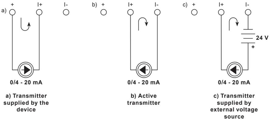
Connection of analog signals 0/4 - 20 mA
