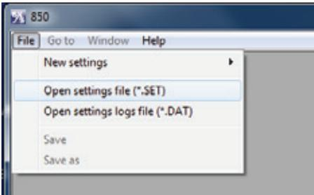
Use the windows operating system to locate and load the desired configuration file.
