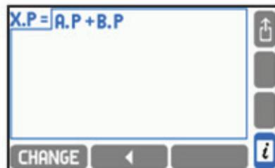
Calculations are performed taking units into account. Formula must have physical sense e.g. density cannot be added to power. Pressures and temperatures are brought to absolute values before calculations. Formula result must be one of physical quantities listed in Section 9.6 or a quantity without unit. If more than one unit is available for the result a proper unit should be taken from a Unit list.
