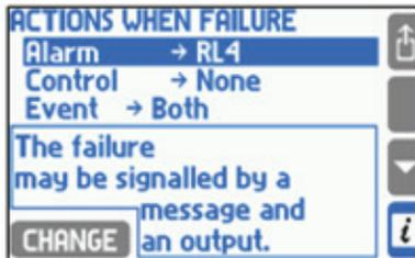
On the selection lists are available only outputs set into proper mode (alarm or control mode). In **Alarm** menu user can choose **Message** only, without relay output assignment. In this case an event will be signaled only by a message and ALARM diode on the front panel and no relay output will become active.
