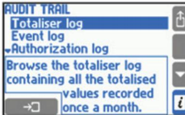
After selecting the totaliser log, the device displays a list of dates and times of available entries. The user should select the right entry and application, then device displays the symbols and states of totalisers in the list.
