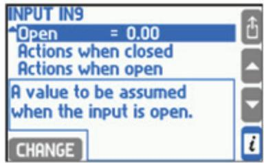
A process value assigned to the binary input in the state monitoring mode may have two values: one, when the input is closed and the other when it is opened (e.g. input closed equals -6.25, and opened +12.5). Both values can be entered in settings. This mode is available only for the inputs with auxiliary values assigned and can be used for indication of flow direction, as a multiplying factor in sophisticated applications.
