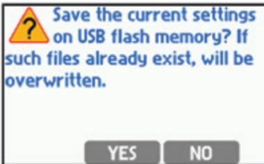
Two files (text and binary) will be created. Text file (extension .txt) allows to read settings on a PC computer using a typical text editor. Binary file (extension .set) enables to load settings to the same or the other device in the future. File name are generated automatically and contains device's RS-485 network address, e.g.: 'sett\_01.txt' and 'sett\_01.set'. If files with these names already exist, they are overwritten. Files names created automatically can be changed only in PC computer.
