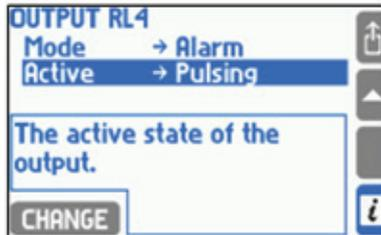
An active state may be closing, opening or pulsing (for alarm mode).
