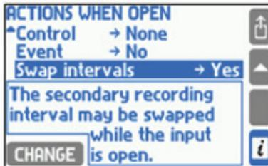
If the second archive speed is not used it is recommended to set it equal to the first one. This is important when using an archive browser in the device because the time scale is selected automatically based on both frequencies.
