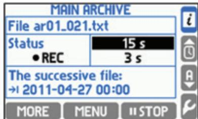
Additional screens are: relay outputs screen, date and time screen and main archive screen. Relay outputs screen informs about status of relays (closed or open, relays not used are not displayed). On date and time screen button **ADJUST** enables setting the clock and calendar. Main archive screen displays information about status of archiving. Bottom buttons enable to control archiving (archive operation is described in Section 10.12).
