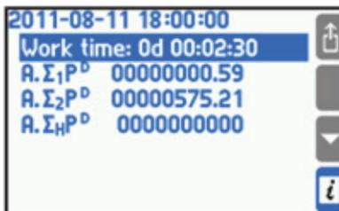
Other logs are displayed in form of a scrolled list. Each line corresponds to one record (event or action). Simultaneously on display there are visible three records. In a frame underneath, additional information about highlighted record is displayed.
