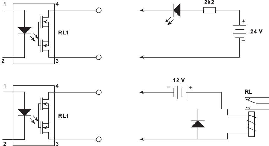
**Connecting the receivers to the binary outputs**
