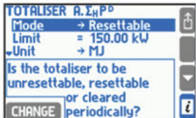
The main  $\Sigma 1$  and the auxiliary  $\Sigma 2$  totaliser add flowrate or heat values in one second periods. An exception is when process value is assigned to binary input operating in pulse counting mode. Then totalisers count pulses multiplied by their values.
