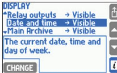
In **Auto interval** submenu time for single screen presentation during automatic scrolling is set. The last three items allow to activate or hide auxiliary screens: relay outputs screen, date and time screen and archive screen. The main screen and individual submenus are set for each application separately. The last submenu item **LCD Display** allows to access the display settings menu.
