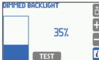
User can set the Background colour as a White or Black. The Backlight can be dimmed when keyboard is not used or can stay always on. The level of backlight can be adjusted in range of 50..100% and the dim level can also be set to 0..45%, both with step 5%. The lower backlight level saves the energy and increases the lifetime of the display.
