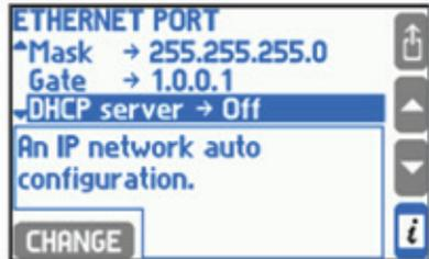
For successful communication between the device and the supervisory system all needed parameters have to be configured (menu: Settings → Ethernet port).
