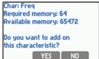
For this purpose in **Char** submenu user should choose **From file....** This will display a list of available files and it allows to add a characteristic table.
