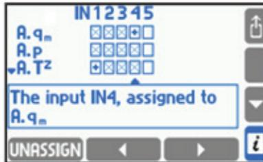
Rows in the table correspond to process values and columns to inputs. Symbol + in the check box means that a value is assigned to the input. X in the check box means that the assignment is impossible. To change the assignment state user has to place a cursor on the check box using arrows buttons and press **ASSIGN** or **UNASSIGN** button.
