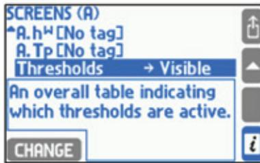
**Main screen** item opens the submenu where are configured the contents of the tables of the main screen of specific measuring application, see Section 10.16.1. Next menu items allow to set detailed screens for process values (resolution of displayed value, range of diagrams and bargraphs and setting visible/hide detailed screens), see Section 10.16.2. The last item **Thresholds** allows to present a thresholds screen.
