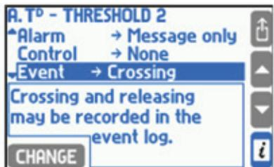
To activate a threshold the first has to be selected the mode (Upper or Lower), and then the threshold value and the hysteresis value. Upper threshold activates when the value exceeds the threshold level and releases when the value declines below that level by at least as much as hysteresis. Lower threshold activates when the value declines below the level and releases when the value exceeds that level by at least as much as hysteresis.
