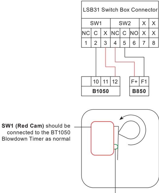
**SW1 (Red Cam)** should be connected to the BT1050 Blowdown Timer as normal
