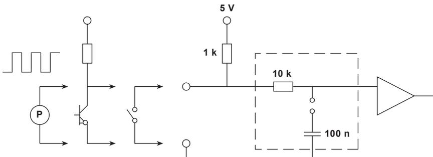
Signal forming circuit for PULS type inputs
