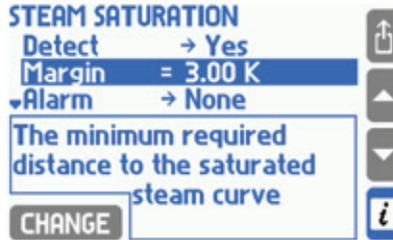
Example: Steam detection was activated and required margin was set to 3.0 K. Steam measured pressure is 1.7 Mpa – at this pressure steam gets saturated in temperature about 204.3 °C. The device will detect steam saturation when its temperature falls down below 207.3 °C (= 204.3 °C + 3.0 K). When temperature grows 0.5 K above this value i.e. to 207.8 °C (= 204.3 °C + 3.0 K + 0.5 K) the device will assume that saturation state is over.
