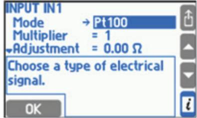
When button **CHANGE** is pressed after selecting a numerical setting the blinking cursor moves to the first digit or the sign of the number that is being changed.
