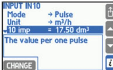
Pulse counting is chosen if a flow meter with a constant pulse value is connected to the binary input. The pulse value should be entered giving a flow value corresponding to the relevant number of pulses. Flowrate value is computed based on measured frequency while the main ( $\Sigma 1$ ) and additional ( $\Sigma 2$ ) totalisers count input pulses multiplied by entered pulse value. In this way no pulse is lost even if a cut-off value is set for flowrate.
