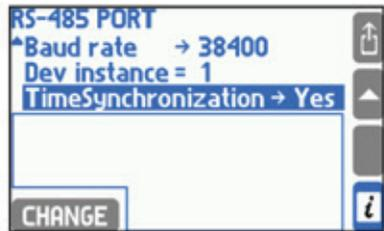
Communication can be done in three protocols (**Protocol** submenu): **ASCII**, **Modbus RTU** and **BACnet MSTP**. ASCII protocol is dedicated for communication with programs delivered by a manufacturer. Modbus RTU protocol serves for communication with universal visualization programs and enables readout of all process values and totalisers. Protocol details are described in Sections 13 and 14. BACnet MSTP provides a data communication protocol for building automation and control networks.
