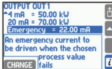
An activation of an output requires assigning selected process value from the list in Value submenu. In the next two positions are required values of extreme currents: 4 mA and 20 mA. Current signal is always in the range of 3.6...22 mA. For values smaller than 3.6 mA the output current stays at 3.6 mA. Similarly for current over 22 mA the output current stops at 22 mA.
