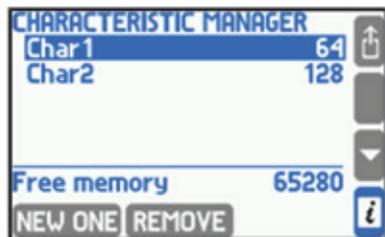
To add on a new characteristic the USB Flash Memory containing a relevant file has to be inserted. In Characteristic manager menu user has to press **NEW ONE** button. A list of files with .txt or .csv. extensions will be displayed and the highlighted file can be chosen with the **LOAD** button. A new characteristic can also be added during the input configuration without need of entering the characteristic database.
