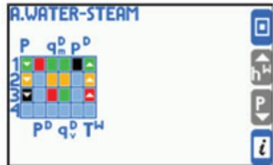
Range of bargraph and trend diagram can be set separately for every value. Range of horizontal and vertical axis of **Trend graph** are displayed after pressing button
