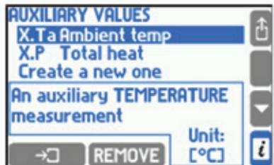
To add a new auxiliary value **Create a new one** function must be chosen and a type of the value and its symbol must be defined. A new item with the new value's setting will be added to the menu.
