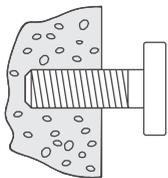
Mounting screw left proud of surface to slot top mounting of B850 over.
