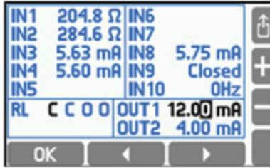
Then insert the value using **+** and **-** buttons, and then press the **OK** button. To restore normal operating of 4-20 mA outputs press **OUT1** or **OUT2**.
