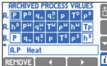
The first two menu items are to select the two archiving speeds(frequency). In normal operation the **Rec interval I** is used. **Rec interval II** may be swapped for the time of alarm and control thresholds activation or for time of closing or opening of output relays. Change of frequency of the recording by a given threshold or output relays must be declared in its setting - **Swap intervals** item.
