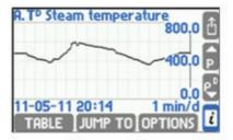
The scope of the presented time interval is dependent on the frequency of archived results (influenced by both of the frequency I and II) and cannot be changed while viewing.
