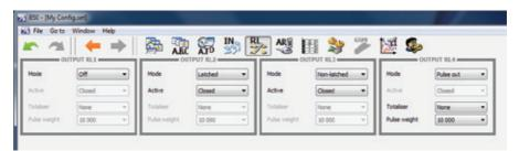
Four relay outputs can be configured.
