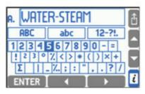
Horisontal and vertical arrow buttons move cursor along the whole screen. Left bottom button, depending on cursor position, can insert or delete a mark from edited text or change set of characters on keyboard. Button is used to leave edition confirming a new text description. There is no possibility to interrupt edition and return to previous text.
