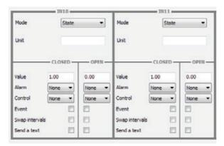
PULS - type inputs: IN10, IN11 and IN12 may be set as '0' volt contacts for automated TDS Blowdown and Bottom Blowdown systems. Ensure voltage does not exceed 40 V.
