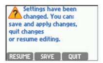
When SAVE button is pressed device operation is interrupted for a few seconds. Then the device resumes with the new settings. Pressing QUIT button denies all changes that were made. Pressing RESUME allows to continue edition of settings.
