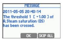
After confirming the message (by pressing button) the output becomes deactivated. Red ALARM diode stops pulsing but it remains on until the event disappears. If another event occurs before confirmation of the previous message then its message is displayed after confirmation of the previous one even if the new event itself disappeared to that moment. The output becomes deactivated after confirmation of the last waiting message. SUP ALL button is used to confirm all waiting messages at one time.
