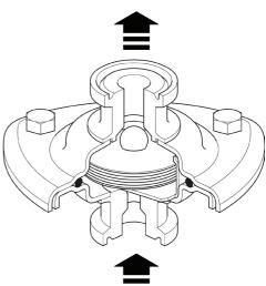
Fig. 1b Sanitary clamp ended variant
