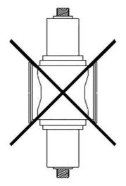
Fig. 12 No vertical alignment of the sensor assemblies
