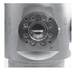
Fig. 19 Armature DTF with window ring FL59 - 8M5 of 90° detector arm
