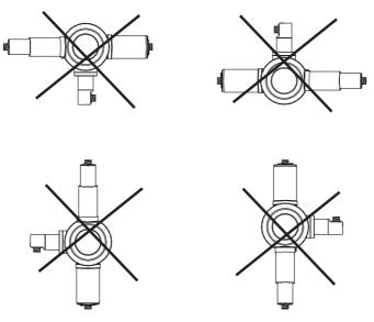
Fig. 16 No vertical alignment of the optical arms
