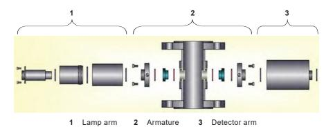
Fig. 1 Exploded view, example: sensor AF26
