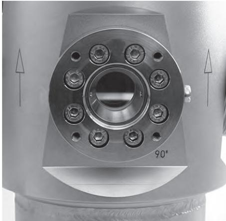
**Fig. 19 Armature DTF with window ring FL59 - 8M5 of 90° detector arm**
