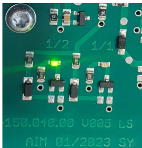
A single LED indicates that the supercapacitor has reached >50% of charge (>12.3V).
