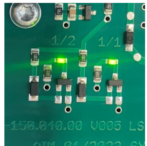
Twin LEDs indicate that the supercapacitor has reached full charge (>20.6V) and is operational.
