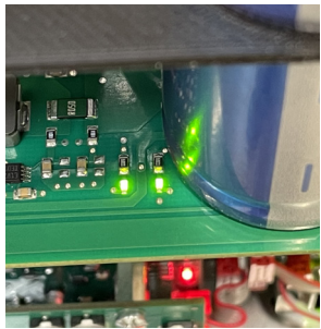
The second bank of LED indicate the state of charge. A single LED indicates >50% charge (10.3V). Both LEDs illuminated indicates 100% charge (>20.6V).
