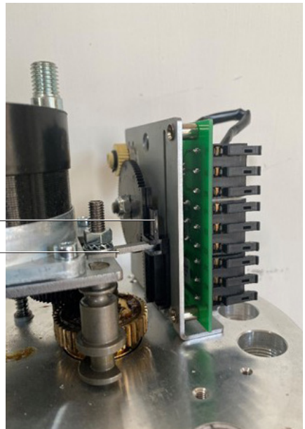
Fig. 8 Auxiliary Travel Switch (WE) Feedback Arrangement (1-6 kN)
