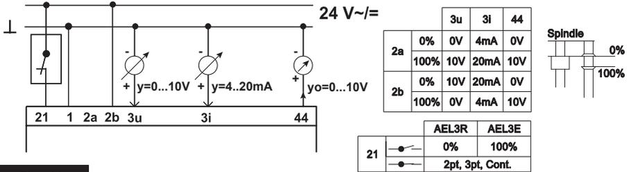
**Fig. 16** Signal to retract actuator
