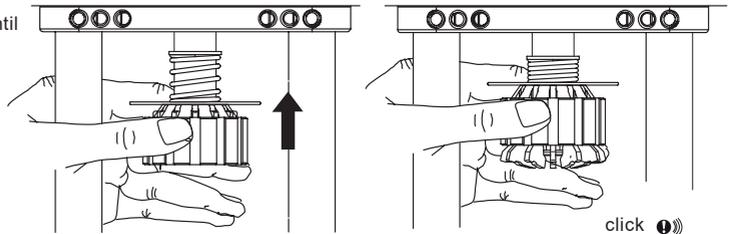
5. Make sure that the spindle is fully retracted into the actuator and handle is up so that the spring is secured in place.
