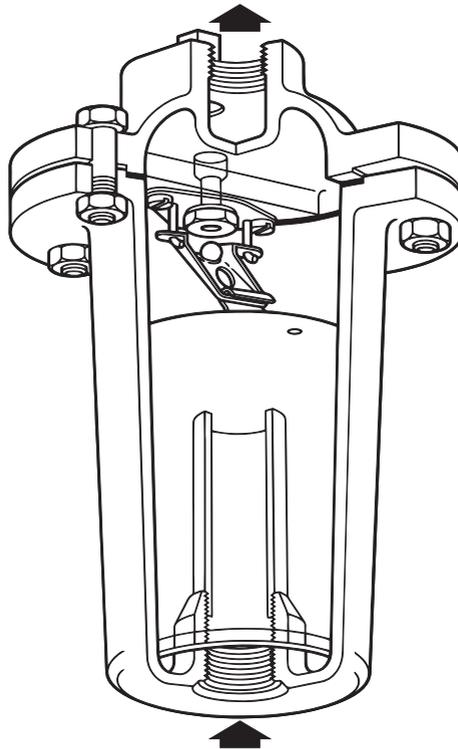
**Fig. 1 200 Series screwed trap shown**
