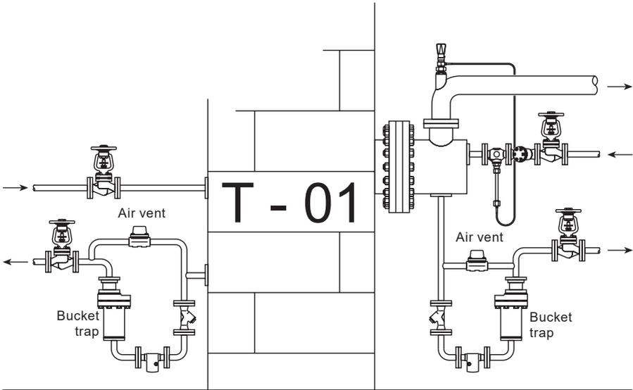
Fig. 3 Typical installation - Oil storage tanks
