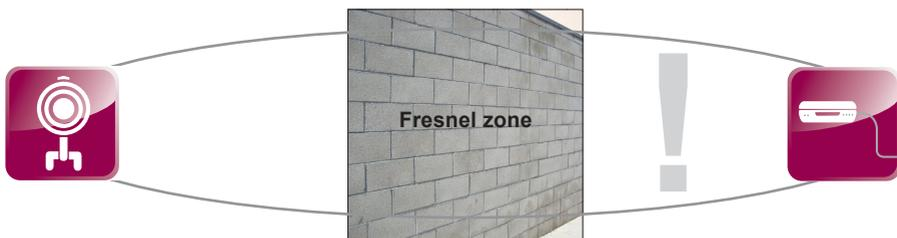
**Fig. 6 Fresnel zone with blockage (obstacle) - Bad**
