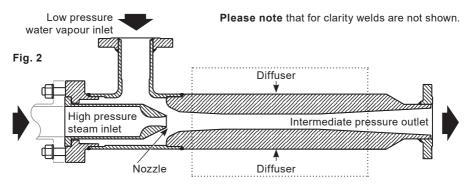
To summarise, high pressure motive steam entrains lower pressure water vapour and, the mixture is discharged at a pressure with a value lying between the suction and motive pressure. In some operating circumstances, the required operating duty of the Thermocompressor can be constantly changing. Thus the amount of motive steam actually required to make the Thermocompressor perform is constantly changing too.
