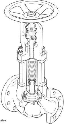
Fig. 1 BSA3HP bellows sealed high pressure stop valve
