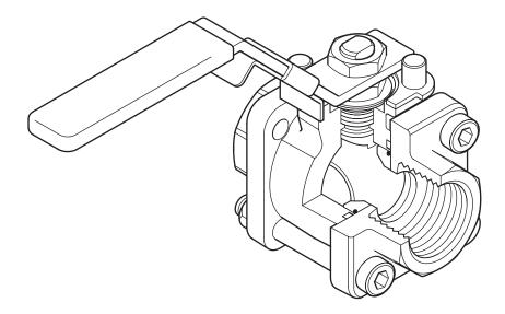
**Description**The M10HPi ISO three-piece body ball valve has a lockable handle and ISO mounting as standard. It features a special floating ball, which has received a surface hardening and a blow-out proof stem. This particular ball valve has been specially designed for manual isolation of applications using high-pressure gas. The M10HPi ISO has been designed for use as an isolating valve, not a control valve, and can be serviced without removal from the pipeline.
