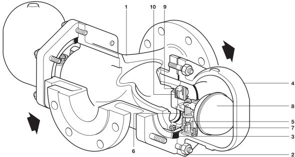
**Description** The FT44 is a carbon steel ball float steam trap with integral automatic air venting facility. It is available with horizontal flanged connections only. If required the covers can be drilled and tapped 2" BSP or NPT for the purpose of fitting drain cocks.
