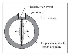
Passage of a vortex causes a slight bow of a wing placed downstream of the bluff body. The bend is measured by a piezoelectric crystal sensor in contact with the top of the wing.
