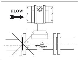
Align the bolt holes of each set of mating flanges. The bolt holes should be directly opposite each other in order to minimize any stress on the flowmeter body.
