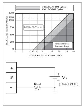
**Analog Output** (JP1 installed or no jumpers) Scalable 4-20 mA output, 2 wire principle. A load resistor may be installed on the supply or return line. Permissible load resistance values are shown in the graph.
