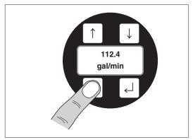
There are two ways to access the interface map from the keypad. The first is to remove the condulet cap, and depress the membrane keys using your fingers.
