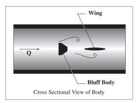
The Vortex S-PhD measures volumetric flow rate by detecting the frequency at which alternating vortices are shed from a bluff body inserted into the flow stream. These vortices are known as Von Karman vortices. The Vortex S-PhD calculates the flow velocity using the following equation:
