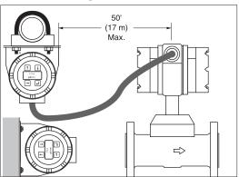
If the temperature of the medium and/or the ambient temperature exceeds the parameters of the shaded area of the graph shown, remote mounting is necessary. There are two options for remote mounting, pipe or wall. The distance between sensor and the electronics must not exceed 50'. If remote mounting is ordered, mounting clamps and plate, and 33' of cable is supplied (50' of cable can be ordered as an option.)
