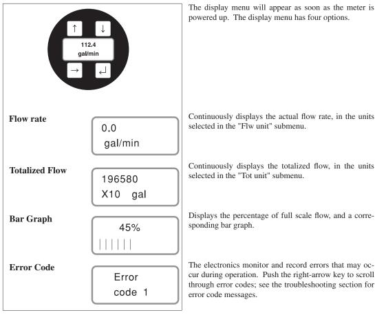
ACCESSING PROGRAMMING SUB-MENUS must hold down the right-arrow key for 2 seconds; then enter the correct password to access the submenus. If the correct password is entered, the display will read "Full Access." If an incorrect password is entered the display will read "Read Only," and the user will not be able to alter any programming.
