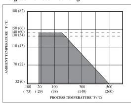
Sensor and electronics can be mounted either integral or remote. For integral mounting, the temperature of the medium and/or the ambient temperature must be within the shaded area of the graph shown . It is possible to shield the electronics from the high temperature of the piping system with thermal insulation blankets.
