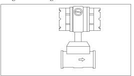
Sensor and electronics are mounted as one unit.
