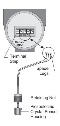
Sensor removal for a remote installation is the same as the integral installation with the following exceptions: 1) the sensor is disconnected from the remote mount condulet on the sensor body instead of at the remote electronics, and 2) the sensor is connected to a terminal strip in the remote mount condulet with spade lugs instead of a female connector.
