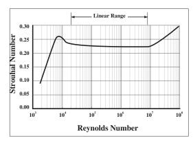
The linear range of the flowmeter (where Strouhal number is constant) is for Reynolds numbers between 20,000 and 7,000,000. (The Strouhal and Reynolds numbers are dimensionless and characterize the flow conditions.)
