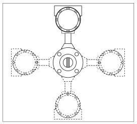
Meter can be installed at any angle.
