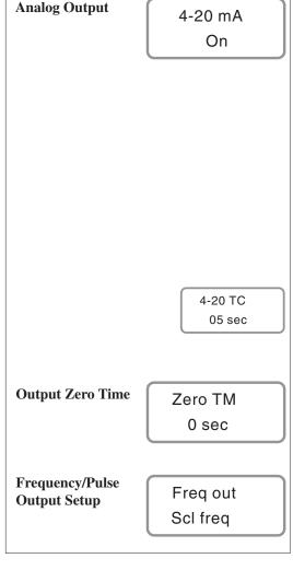
Linear analog output set by min. and max. flow. Toggle on/off with the up and down-arrow keys.
