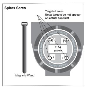
The second method is to use the magnet wand. This allows the keys to be activated through the condulet cap, and is required to maintain the explosion proof rating.
