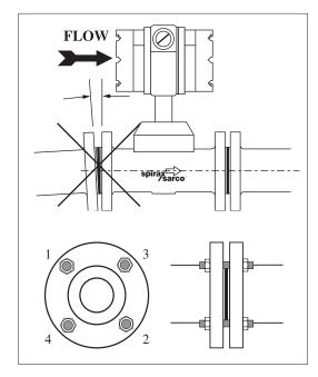
Snug all bolts prior to final tightening. Tighten bolts in a staggered fashion to avoid tilt.
