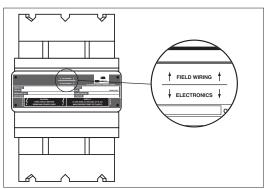
The field wiring terminal for power and signal wiring may be accessed by removing the field wiring condulet.
