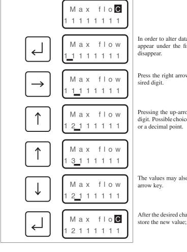
In order to alter data, press the enter key. A cursor will appear under the first digit. Note: blinking icon will disappear.
