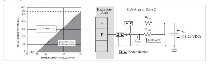
The Vortex S-PhD flowmeter may be operated using a 24 VDC power supply. The 4-20 mA output is scalable (2 wire principle). Permissible load resistance values are shown in graph. The pulse output should be connected to a high impedance, electronic counter.
