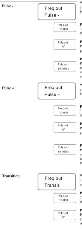
With this output selection, one negative pulse is generated each time the totalizer increments. The increment is set by the Per pulse and pulse unit.
