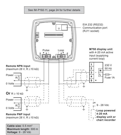
**Important:** Cable type for both loop and pulse **must be** shielded twisted pairs, each core, seven stranded wire with cross sectional area of 0.5 mm<sup>2</sup>
