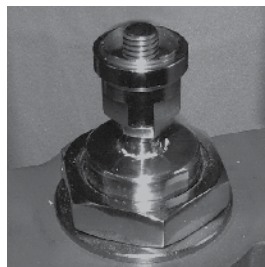
Fig. 18 Incorrect - thread protruding above the adaptor
