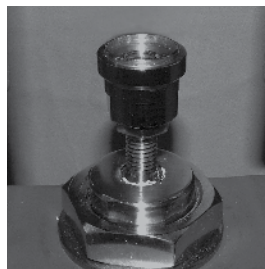
Fig. 17 Correct - 8 mm thread engagement
