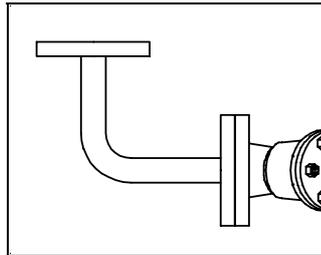
You will see that the pipework has been completed and that a 32mm/1¼" flange has been added ready for the next product to be attached.
