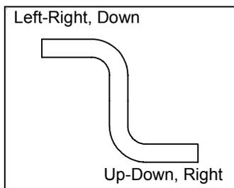
On this occasion **Left - Right, Down** and **Up - Down, Right** pipework have been connected together. The end-caps are removed automatically.
