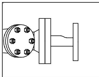
The reducer should look like this when inserted. The outlet is now 15mm/½"
