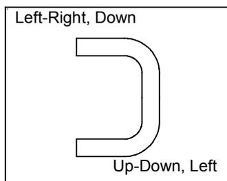
On this occasion **Left - Right, Down** and **Up - Down, Left** pipework have been connected together. The end-caps are removed automatically.
