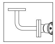
You will see that the pipework has been completed and that a 32mm/1½" flange has been added ready for the next product to be attached.
