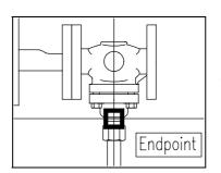
Use *Endpoint* to connect the actuator to the valve
